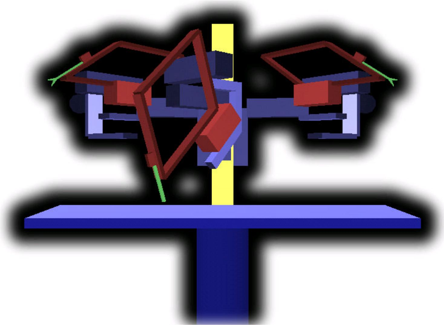
The visualizer is also capable of rendering an image from the perspective of the camera, mounted on the third arm of the “da Vinci” system. The following screenshots demonstrate the “third-person” and “first-person” views of the robot; a highlighted area is provided to clarify the perspective.
